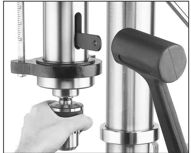
Figure 32. Using drift key to remove arbor.
