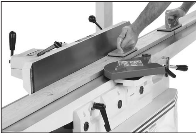
Figure 34. Example of surface planing operations.
