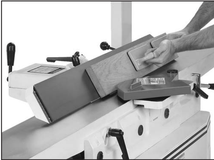
Figure 38. Fence setup for a bevel cut of 45°.
