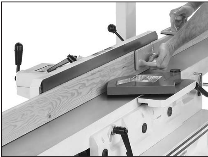
Figure 36. Example of edge jointing operation.
